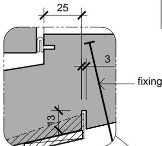
**Alternative Sill Flashing For Timber & Concrete**
